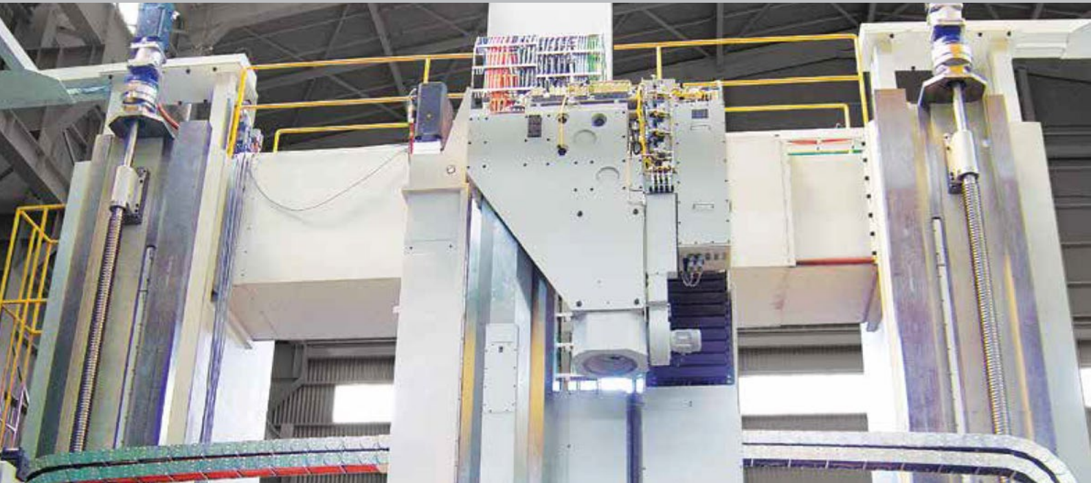
Crossrail moving and synchronization
